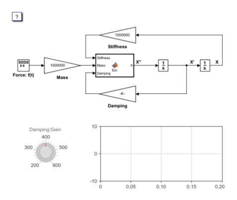
The model implements a second-order physical system called an ideal mass-spring-damper system. Gain blocks represent components of the system equation: Mass,
